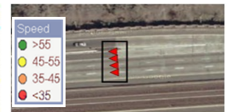
Figure 3. S_D map of detector speeds (MPH) at 10:50 AM on Feb 5, 2008. The black box shows the incident region.
