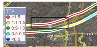
Figure 2. S_L map of I-66 link-level travel time index (TTAi) at 10:50 AM on Feb 5, 2008. The black box shows the incident region.
