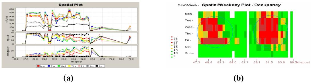
**Figure 5.** Shows speed, volume, and occupancy of a set of station nodes for a specified time of day
