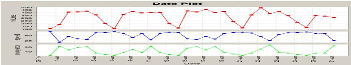
**Figure 2.** Shows speed, volume, and occupancy of a particular station for a specified date range
